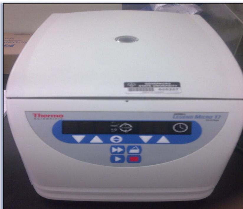
**Figure 7:** Thermo scientific Sorvall Legend Micro 17 Ventilated micro centrifuge with 24 place rotor, 120VAC (8898 RPM for 12 minutes)
