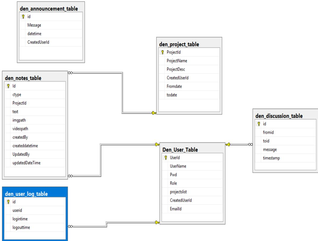
The above screenshot displays completely about the Database tables and ER diagram where DEN is the database name.
